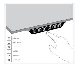
The height is adjusted by pressing 2 buttons (arrows up and down). The height adjustment controls are provided with a 3-position memory, which allows you to program up to 3 heights.
